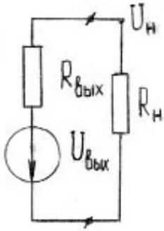
$$U_{\text{H}} = \frac{U_{\text{ВЫХ}}}{R_{\text{ВЫХ}} + R_{\text{H}}} R_{\text{H}} = U_{\text{ВЫХ}} \xi_{\text{ВЫХ}}$$
