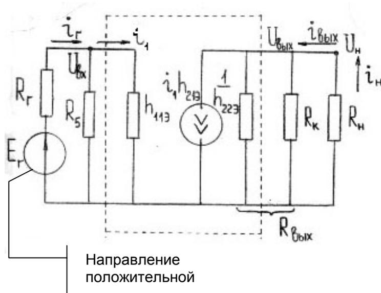
$$R_{вх} = \frac{U_{вх}}{I_{вх}} = \frac{U_{вх}}{I_r} = \frac{i_1 \cdot h_{11э}}{\frac{i_1 \cdot h_{11э}}{R_б} + i_1} = \frac{h_{11э} \cdot R_б}{h_{11э} + R_б} = h_{11э} \parallel R_б ;$$
