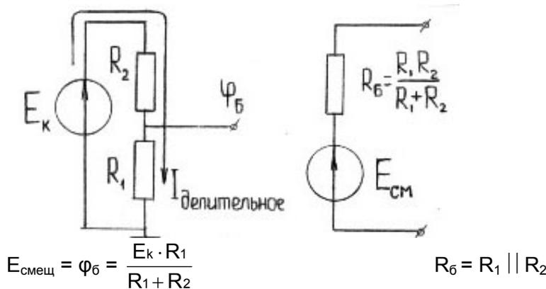
$$E_{смещ} = \varphi_B = \frac{E_k \cdot R_1}{R_1 + R_2}$$
