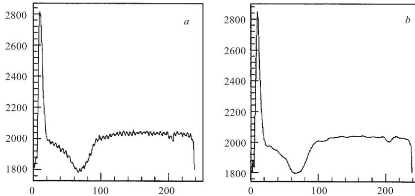
Fig. 3. *a*) One inter-beat interval of raw ECG, *b*) approximation (2) of the same interval
